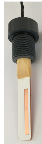
Fig 2 FMRS06 ER Sensor as used in Test 1 & 2
